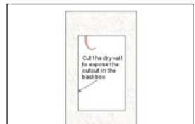
Cut the opening in the drywall to expose the backbox.
