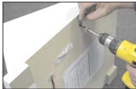
Screw on the supplied hooks.
